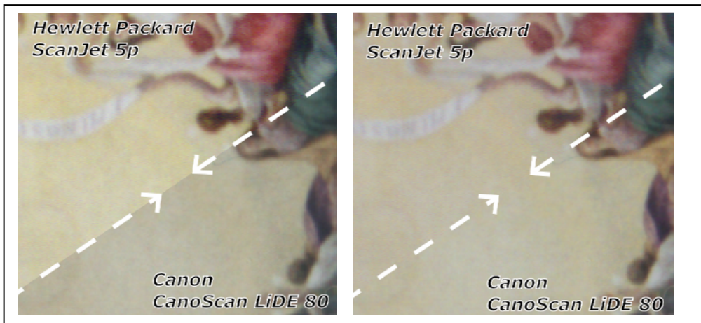
Figure 6: Colour differences of uncalibrated (left) and calibrated (right) scans in detail
