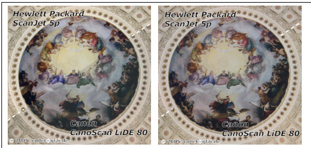
Figure 5: Uncalibrated (left) and calibrated (right) scans of a photo showing the "Capitol Rotunda Ceiling"
